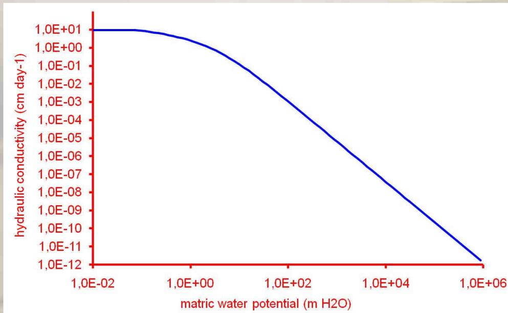
When experimental data of hydraulic conductivity are not available, the SWR is used to derive the hydraulic conductivity curve, which is necessary for solving Richards equation.
